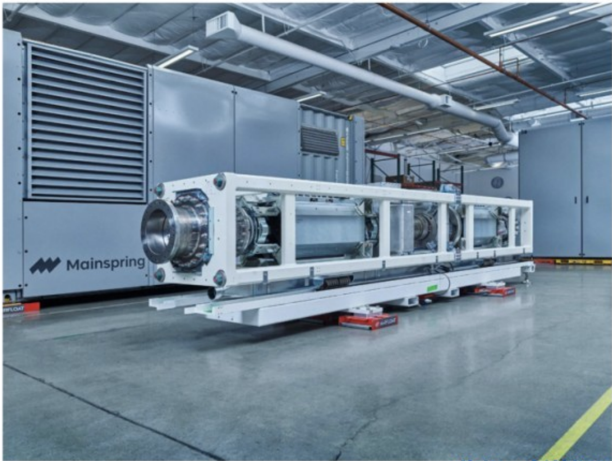
Mainspring Energy's linear generator core at the company's manufacturing facility in Menlo Park, California. Photographer: Spencer Lowell for Bloomberg Green china-nengyuan.com
